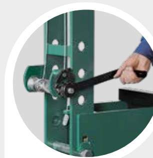
Fast and safe adjustment of the press table height, using a braked winch.
