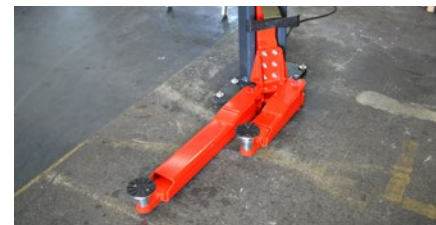
Parallel position of the swivel arms possible, for easier and faster positioning of the vehicles
