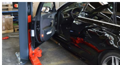
Large door opening angle Door stop protection
