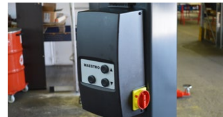
Pushbutton control with possibility to park in safety ratchets
