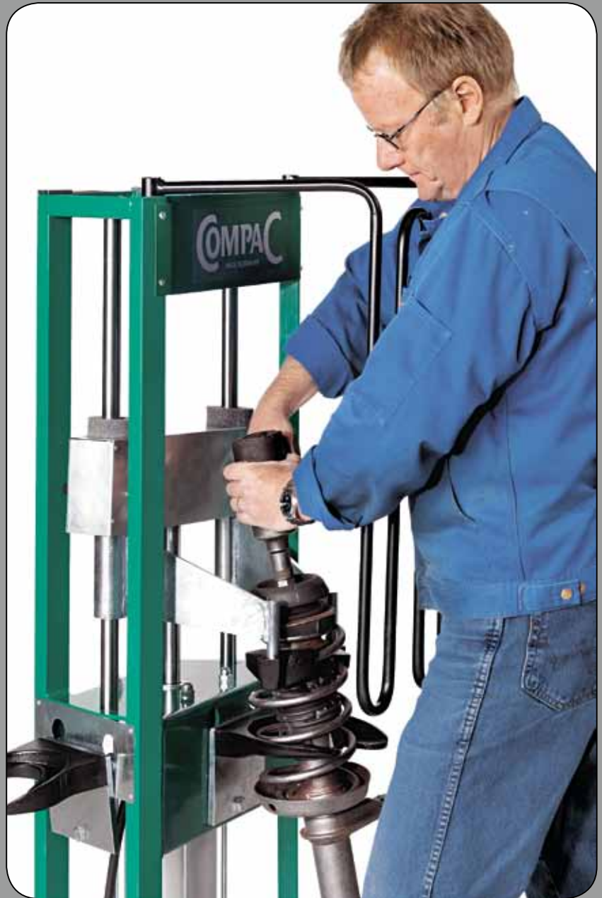
Easy access to mounting and demounting of the top nut.
